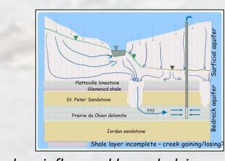
Conceptual illustration of losing and gaining reaches of the creek as influenced by underlying geology. The underlying Platteville-Decorah Shale formation inhibits downward flow, if present
