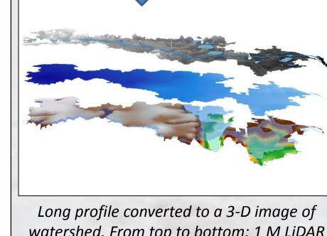
watershed. From top to bottom: 1 M LiDAR surface (MnGeo 2011), water table (surficial aquifer), top of bedrock aquifer, and piezometric surface (Tipping 2011).
