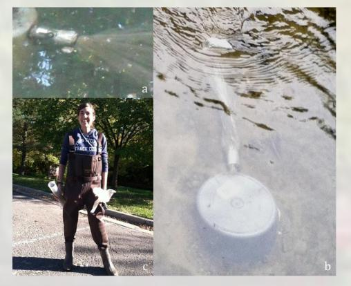
(a) Close-up of hose-fittings used to attach the seepage meter to a plastic bag in which the change in a volume of water over a set period of time is measured. The valve is closed when the bag is removed or attached to avoid losing water. (b) Seepage meter deployed in streambed. (c) Trisha Moore measuring the volume of water in
