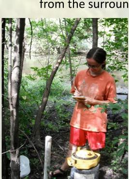
Undergraduate student Laina Breidenbach collecting water level data from one of several installed piezometers throughout the Minnehaha Creek Watershed Water levels were also measured in the creek to determine a stage difference or hydraulic gradient between the creek and surrounding riparian corridor.
