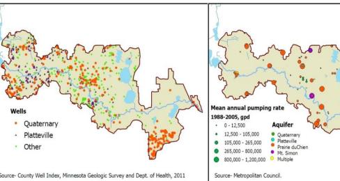
Groundwater pumping locations and magnitude within the lower watershed As noted in the map, large capacity wells are located primarily within the Prairie Du Chien Aquifer. In some areas this aquifer can have a direct connection with Minnehaha Creek.
