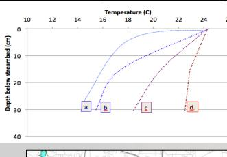
Profiles of (a) high and (b) medium groundwater flux to the creek, (c) no subsurface flux, and (d) surface water flux to surficial aquifer (loss).
