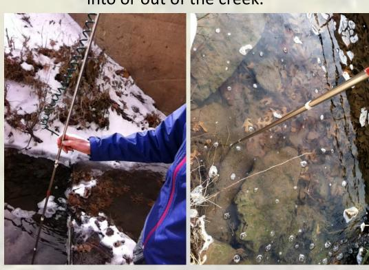
(Left) Six Inch graduations on temperature probe used to determine relative depth within channel sediments. (Right) Insertion of temperature probe into channel bottom sediments. The overall depth of measurements varied between locations and depended on the type of bed material present.
