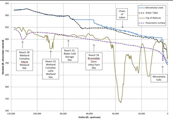
Long profile of surficial and bedrock aquifer systems along Minnehaha Creek. Created using 1 M LiDAR Surface (MnGeo 2011) and subsurface layers from Tipping, 2011.
