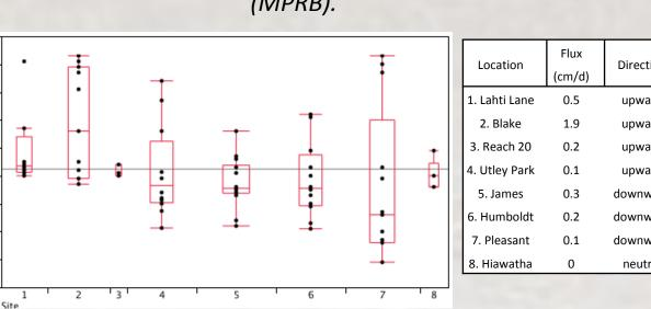
Box plot and table of seepage meter measurements at 8 locations along Minnehaha Creek. Sites are presented in order from upstream to downstream. The gray horizontal line denotes the average flux across all sites (0.2 cm/day upward); average flux rates by site are listed in the table. Flux values less than 0 signify seepage of surface water into the streambed.
