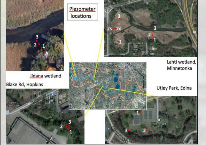
Location of piezometer installations along Minnehaha Creek. Filled circles denote approximate location of piezometers. Piezometers were placed at varying proximities to the creek at each location to better determine the spatial distribution of groundwater fluxes.
