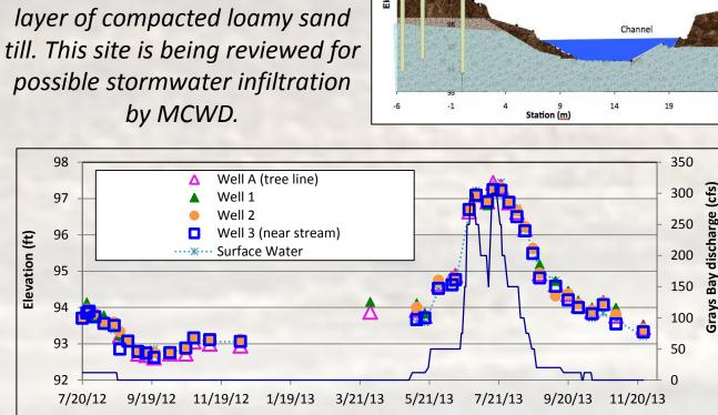
Piezometric head and surface water elevation measurements at the Jidana Park wetland located in the creek's headwaters. Groundwate head is highly correlated with Grays Bay discharge at this site.
