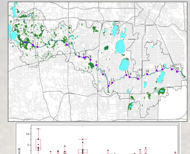
Box plot of groundwater flux as calculated from measured streambed temperature profiles at 20 sites along the length of Minnehaha Creek. Numbered labels in the box plot correspond to numbered locations of temperature probe sites in the map. Positive flux values represent upward groundwater movement; negative flux values denote downward groundwater flux.
