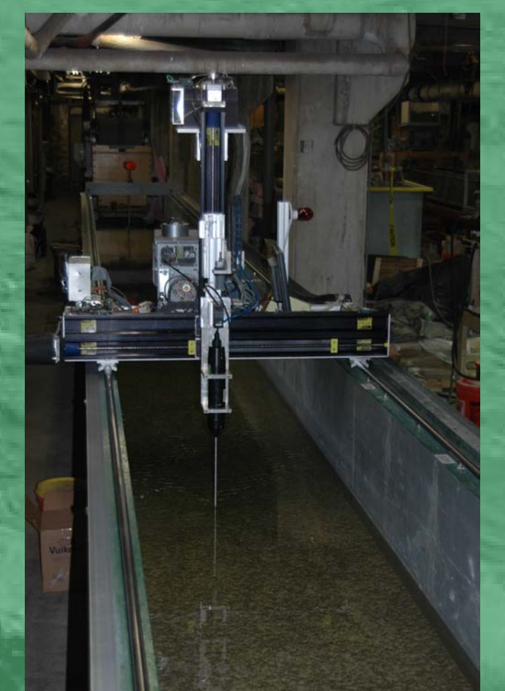
ADV collecting data in the SAFL Tilting Bed Flume
