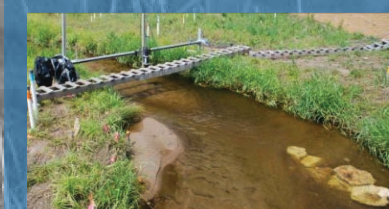
Rock vane in the SAFL Outdoor StreamLab. ADV measurements occurring upstream from the structure.
