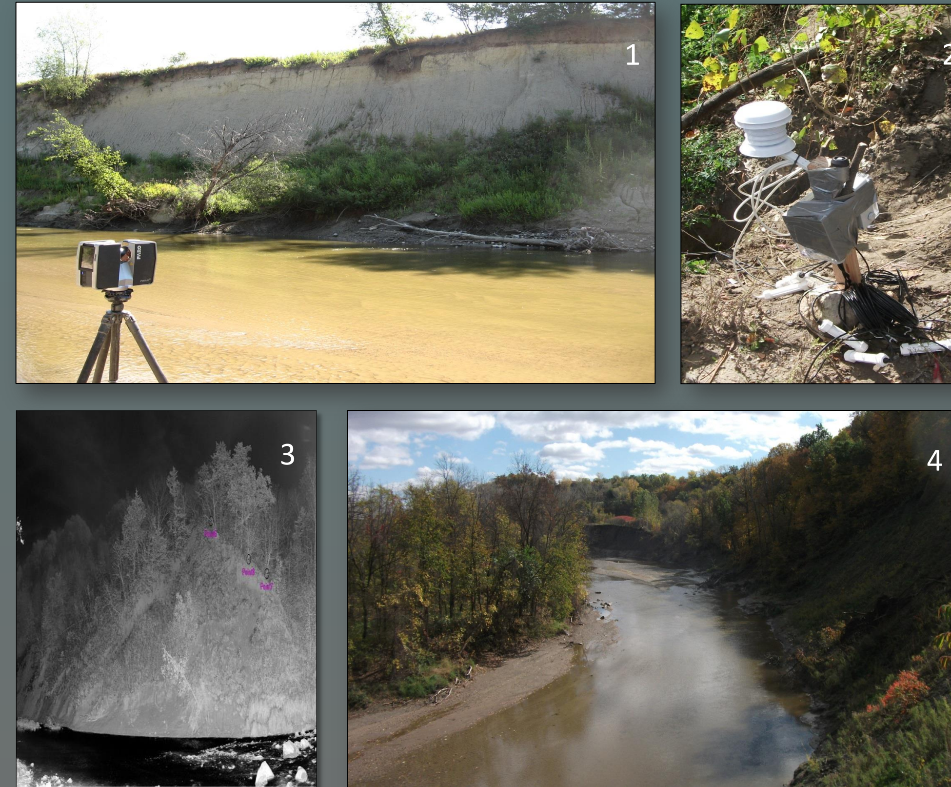
1: Terrestrial Laser Scanner setup for scanning 2: Sensor setup in one of the bluff 3: Point cloud generated after TLS scanning 4: Upstream section of LS-7756 in Le Sueur River
