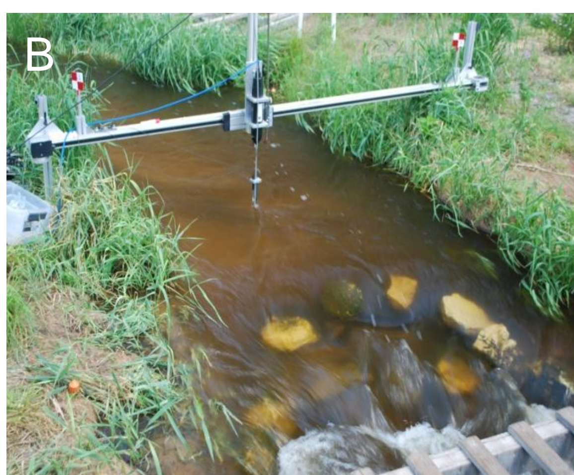
Figure 1: Photographs illustrating A) the bracket system, which holds (from left) the NO x biosensor, DO microsensor, and temperature sensor along with B) the traverse system, which mounts the ADV and allows for transversal and vertical measurements within the stream and near structures (cross vane shown in this photograph). Stream flow is from left to right in both photographs.
