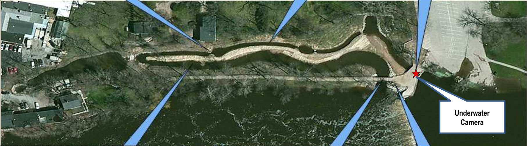
One of eight rock weirs that allow fish to move through the fishway elevation change
